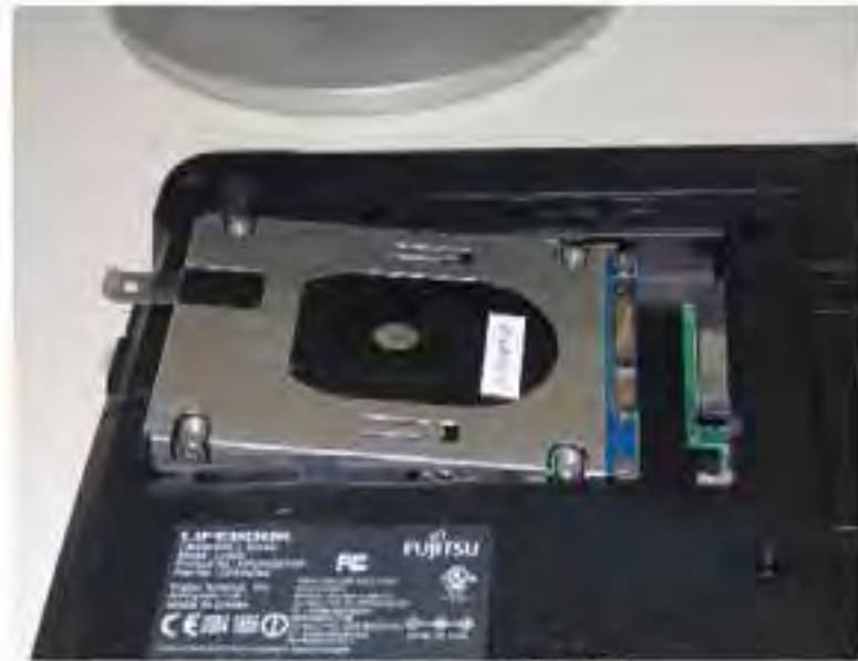
LH531 Removing Old Drive
